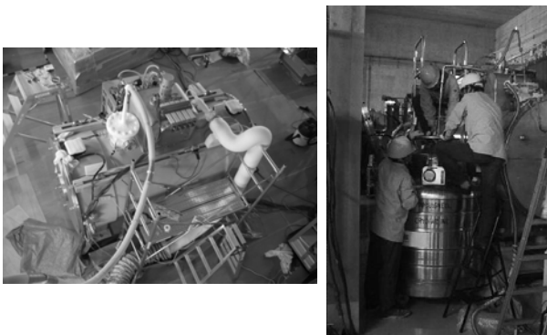
Fig. 1. Precooling by transferring liquid nitrogen (left). Transferring liquid helium from dewar (right).
