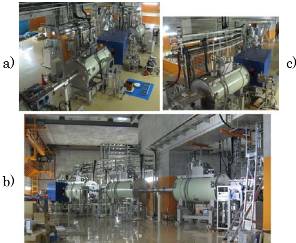
Fig. 3. Photographs of ZeroDegree spectrometer: a) shows a view of the target position, while b) and c) show those of the intermediate and final focuses, respectively.
