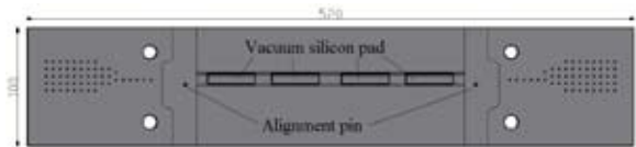
Fig. 1. The stave jig has four bushes. Each pair of diagonal holes is used for the relative position determination of the jigs to be placed properly with pins.
