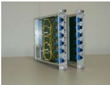
Fig. 3. Photograph of transmitter and receiver modules packaged in NIM module. The left and right components are the transmitter and receiver modules, respectively.
