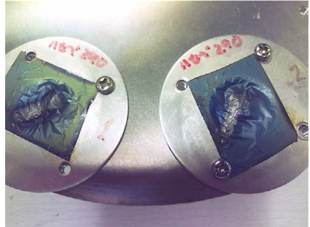
Fig. 2. Photograph of C-foils after the beam irradiation. The left foil was irradiated with helium gas and the right foil was irradiated without gas.
