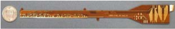
Fig. 3. The final prototype pixel bus prior to attachment of the sensor modules and connectors. The 500 Yen coin provides the scale.
