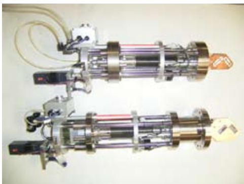
Fig.2. Photograph of emittance monitor systems. The upper part shows a slit system and the lower part shows the electrode system.
