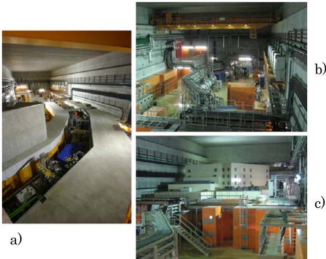
Fig. 2. Photographs of BigRIPS separator: a) and b) show the first and second stages of the BigRIPS separator, respectively, while c) shows the first stage after the thick radiation shields were installed.
