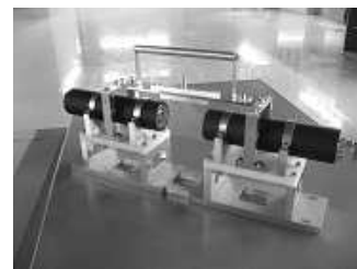
Fig. 5. Outside view of plastic scintillation counter.
