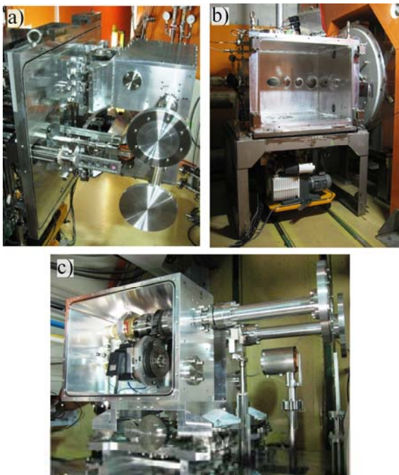
Fig. 1. a) Target flange unit. b) Target vacuum chamber and vacuum pump unit. c) Internal view of the disk target unit containing a motor and water inlet tubes.
