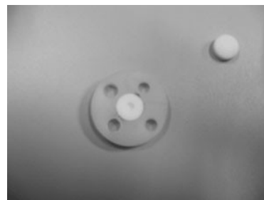
Fig. 2. Holder for collection of short-lived nuclides using a gas-jet transport system.
