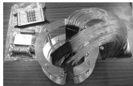
Fig. 2. Picture of multiplicity filter viewed through optical fibers during assembly
