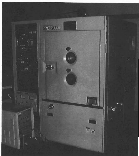
Fig. 1. High vacuum evaporation system (EBX-2000C by ULVAC).
