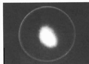
Fig. 3. Positron beam profile observed using the MCP. The MCP active diameter (a ring diameter) is 10 mm.
