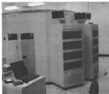
Fig. 2. PowderHorn9310 is one of the largest tape libraries. It can store up to approximately 6,000 cartridges.
