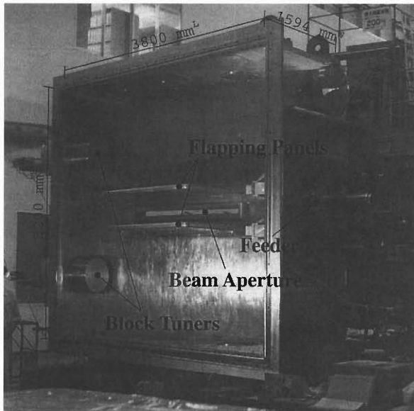
Fig. 1. The IRC accelerating resonator. The side flange on which the dee electrode is attached is removed.
