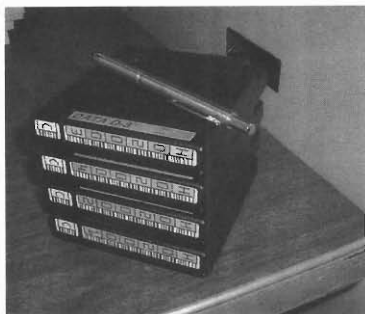
Fig. 1. SD-3 tape cartridge has 50-GB capacity in a small dimension: 100 \times 125 \times 25 mm 3 .
