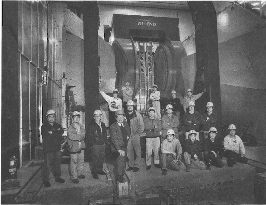
Fig. 1. The PHENIX detector. Two magnets with a flowerpot shape on the left- and right-hand sides are the muon magnets (the left one is fabricated in Kobe, Japan). Adjacent to these, one can see the panels of the muon identifiers. The central magnet and the frames of the central arms are seen at the center, pending the installation of the detectors for electrons and photons. [Photograph by R. Stoutenburgh (BNL)]
