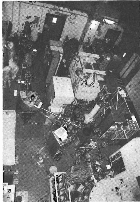
Fig. 1. Photograph of the new injector system along with the beam transport line starting from the existing 450 kV Cockcroft-Walton terminal.
