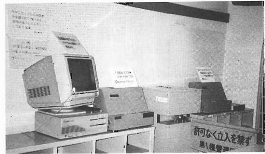
Fig. 1. The photograph of the film badge reading system.
