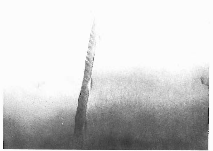
Fig. 1. Bubbles on dislocations in the specimen not heat-treated after irradiation.
