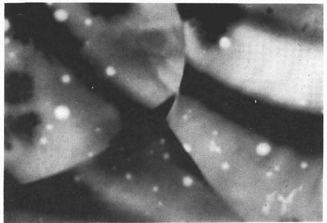
Fig. 3. Bubbles and grain boundaries in specimen A as irradiated. ( \times 50000 )
