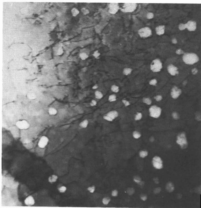
Fig. 4. Sample B annealed for 1 h at 800 °C. All bubbles are attached to dislocation lines.
